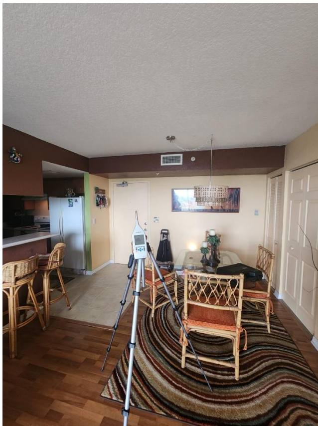
Figure 2; During FIIC measurements in living-room of apt.802
