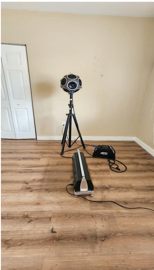
Figure 2; Apartment #210 Room 1, During IIC testing.
